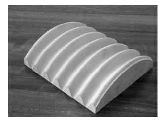
Figure 7: The mould used for vacuum-forming the plastic shell. This was produced on a computer-controlled milling machine.
