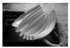
(c) The shell can be inextensibly deformed to a positive Gaussian curvature, (*i.e.* bowl-shaped) or
